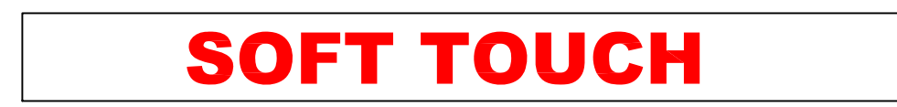
INFORMATIONAL SIGN #07 SCALE: 1/2" = 1'-0" NON-LIT INFORMATIONAL SIGN RED VINYL ON WHITE ALUMINUM 1'-0" H X 10'-0" W = 10.0 SQ FT
