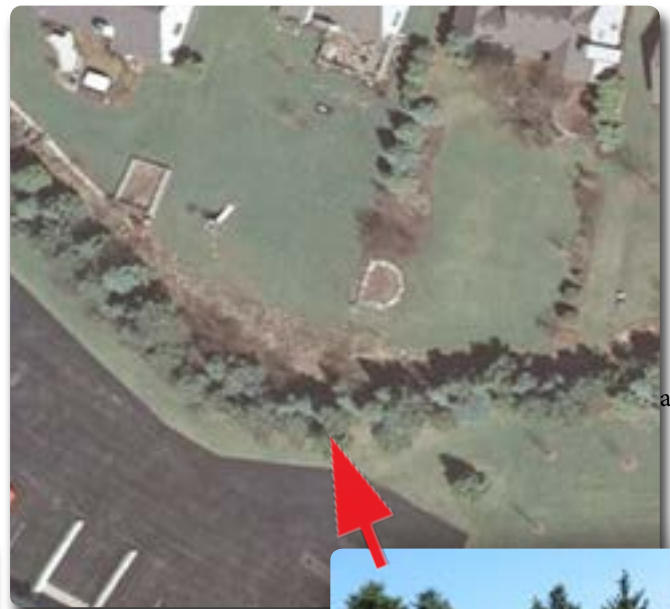
Landscape berm for visual and noise buffering between non-residential and residential developments.
